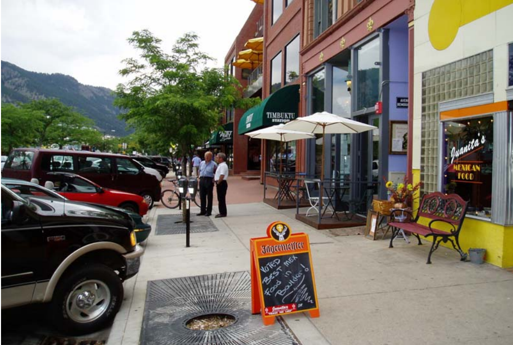
Figure 13: Creating a pedestrian realm in Boulder, Colorado using diagonal parking, planting/furnishing strip, sidewalk, and setback
